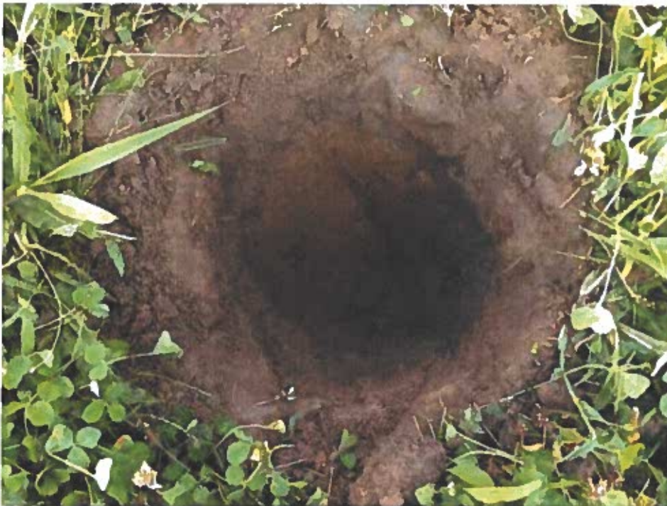
Image 4: Typical Test Pit
